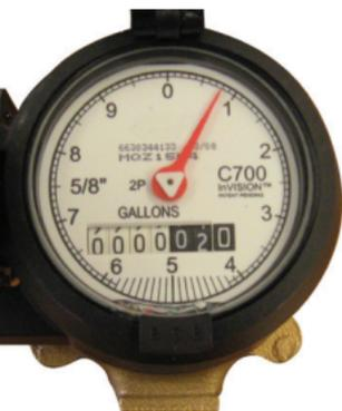
Most meters have some indicator that will spin or revolve whenever water is running. If no water is known to be on, this will tell you if water is flowing through your meter.
